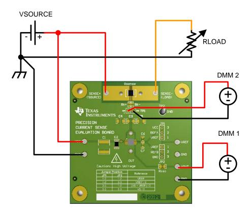
Figure 8: Setup for Uni-Directional Devices
