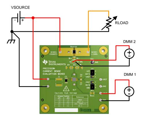
Figure 9: Setup for Bi-Directional Devices
