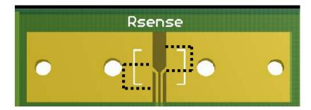
Figure 3: Cutting pads to accommodate 4-wire resistors
