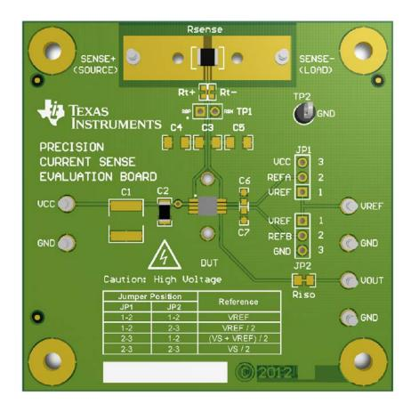
Figure 1: Picture of Evaluation Board (LMP8480 version)
