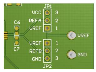
Figure 6: Reference Jumper Pins
